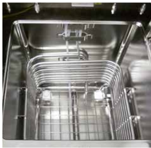
The new processing machine under the name "MEDLINE Clean" cleans contact lenses from residues and subsequently coats the lenses in the course of an additional processing step.
