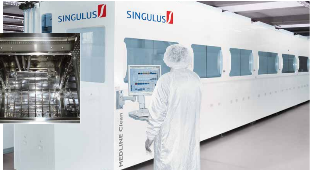
The new processing machine under the name "MEDLINE Clean" cleans contact lenses from residues and subsequently coats the lenses in the course of an additional processing step.
